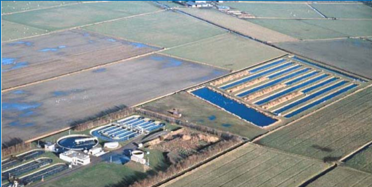
Constructed wetland on the isle of Texel (NL) for further polishing of tertiary treated wastewater and ecological upgrading (Water Harmonica concept) (Toet, 2003)
